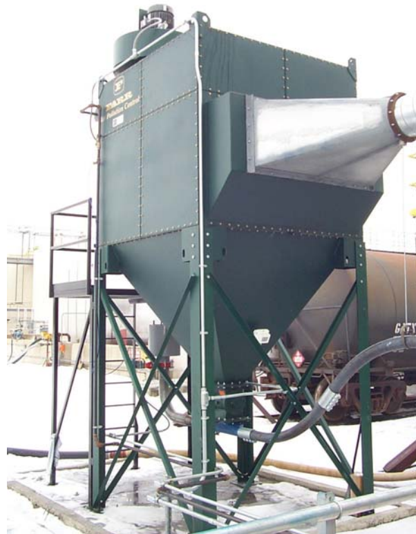
Farr Model GS-16 With 10X10 Air Lock Top Mounted Blower 6000 CFM @ 8" SP Ink Pigment Collection
