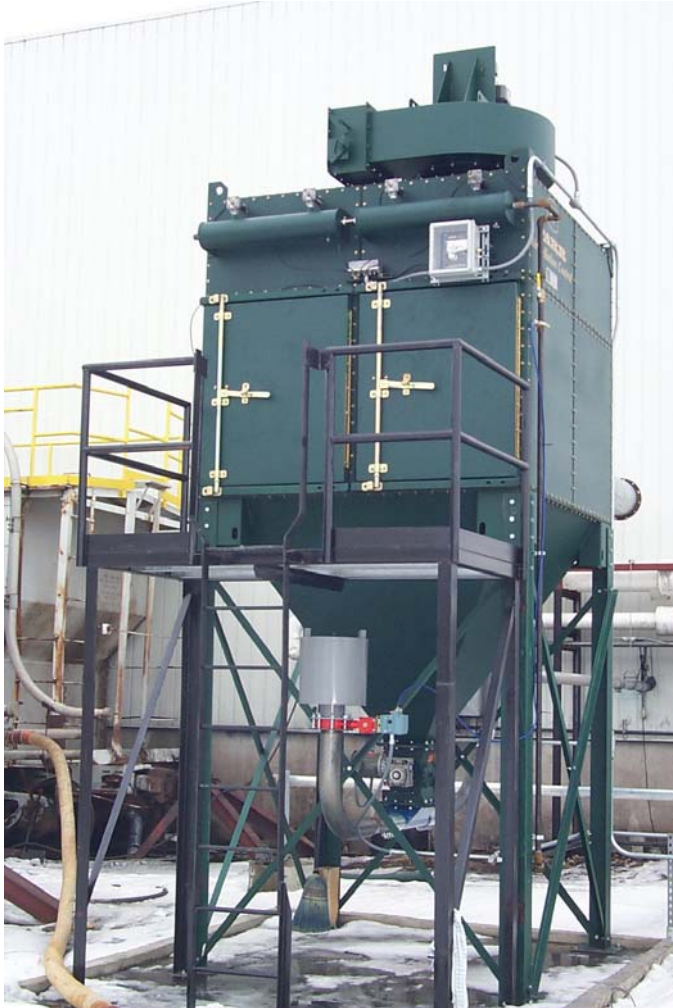
Farr Model GS-16 With 10X10 Air Lock Top Mounted Blower 6000 CFM @ 8" SP Ink Pigment Collection
